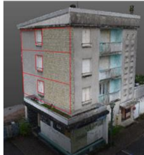
Figure 2. Generation of the module-layout from the Point Cloud coordinates.
